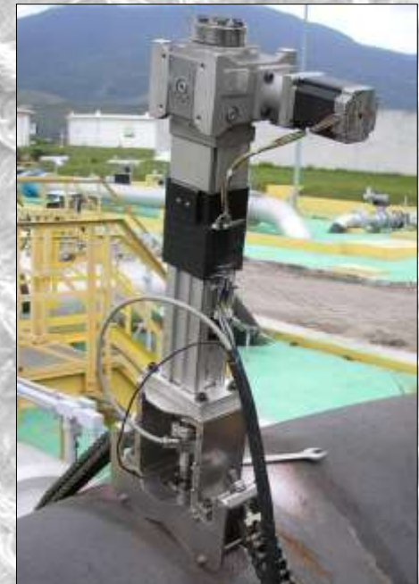
In situ measurement of mechanical properties on an oil pipeline
